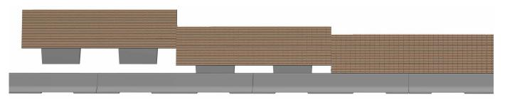
The REBLOC<sup>®</sup> Integrated Noise Barrier consists of a base element of New Jersey profile and a plateshaped noise barrier element. The slim total system width makes optimum use of the space available. One noise barrier element is inserted overlapping two base elements. This configuration enhances stability. The patented coupling system guarantees a high restraint function and connects the elements to a strong chain.
